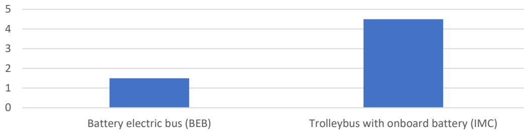
Figure 46: Illustrative daily number of cycles for a battery on a battery electric bus compared to a trolleybus with an onboard battery (in-motion charging bus). Estimation uses the metrics provided by Centrale d’Achat du Transport Public ( Etude-comparative-des-differentes-motorisations-de-bus-2024.pdf ): a battery size of 450 kWh and electricity consumption rate of 125 kWh/100 km for a BEB and a battery size of 50 kWh and electricity consumption rate of 190 kWh/100 km for an IMC bus, an average daily distance of 300 km for both bus types and an estimation of 40% of the IMC bus daily route requiring battery use instead of overhead power supply.
