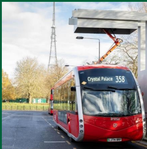
Figure 12: Pantograph charging of a BEB at Crystal Palace in London, UK.
