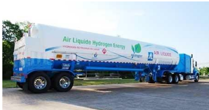
Figure 10: An Air Liquide truck delivering liquid hydrogen 16
