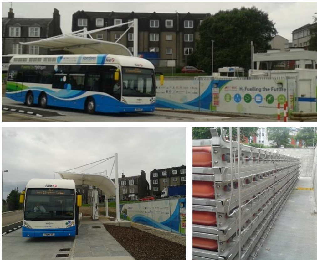
Figure 15: FC bus and hydrogen storage at the Kittybrewster HRS
