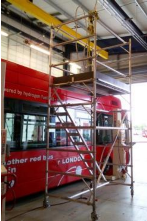
Figure 3: Example of a mobile working platform used in London
